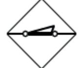
Electronic limiter                               |
