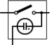
Switch with neon lamp incorporated                 |
