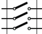
DIP<br>encapsulated switches<br>e.g. 3 switches    |
